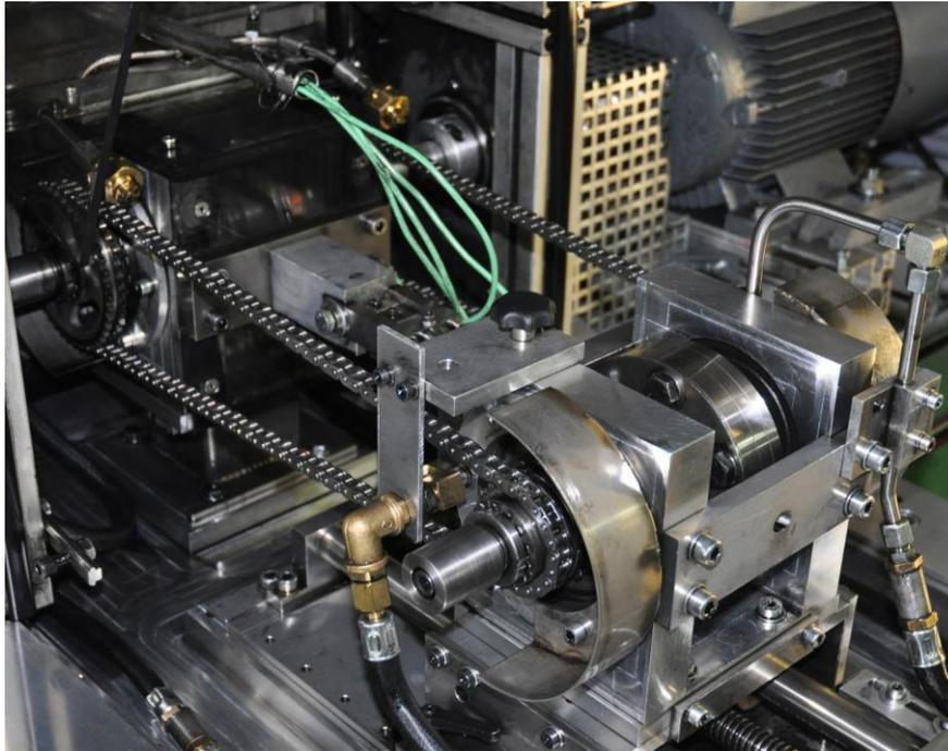
Modular chain wear test rig
