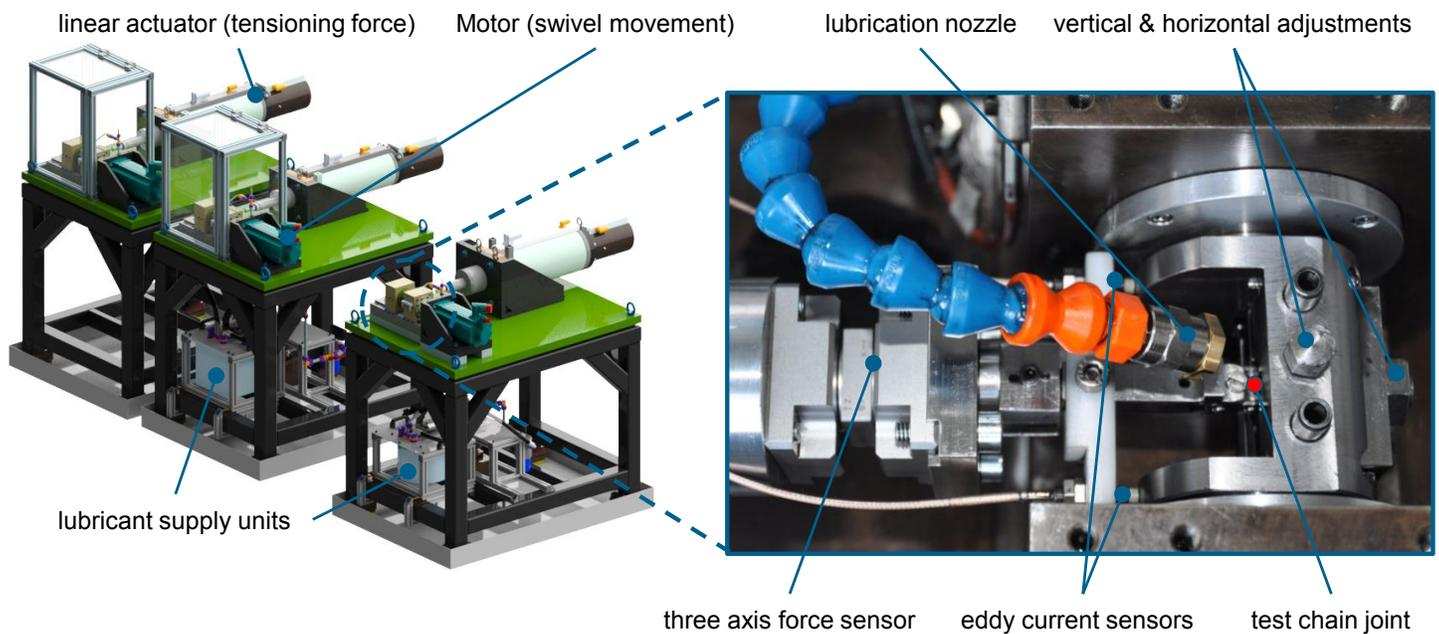
**Figure 1: Chain joint tribometer for friction and wear investigations on single chain joints**
