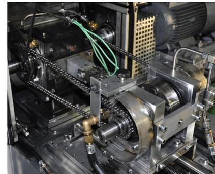
Chain wear test rig
