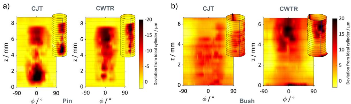
**Figure 3: Results of roundness measurement of pin (left) and bush (right) of chain wear test rig (CWTR) and chain joint tribometer (CJT) after 50h runtime**
